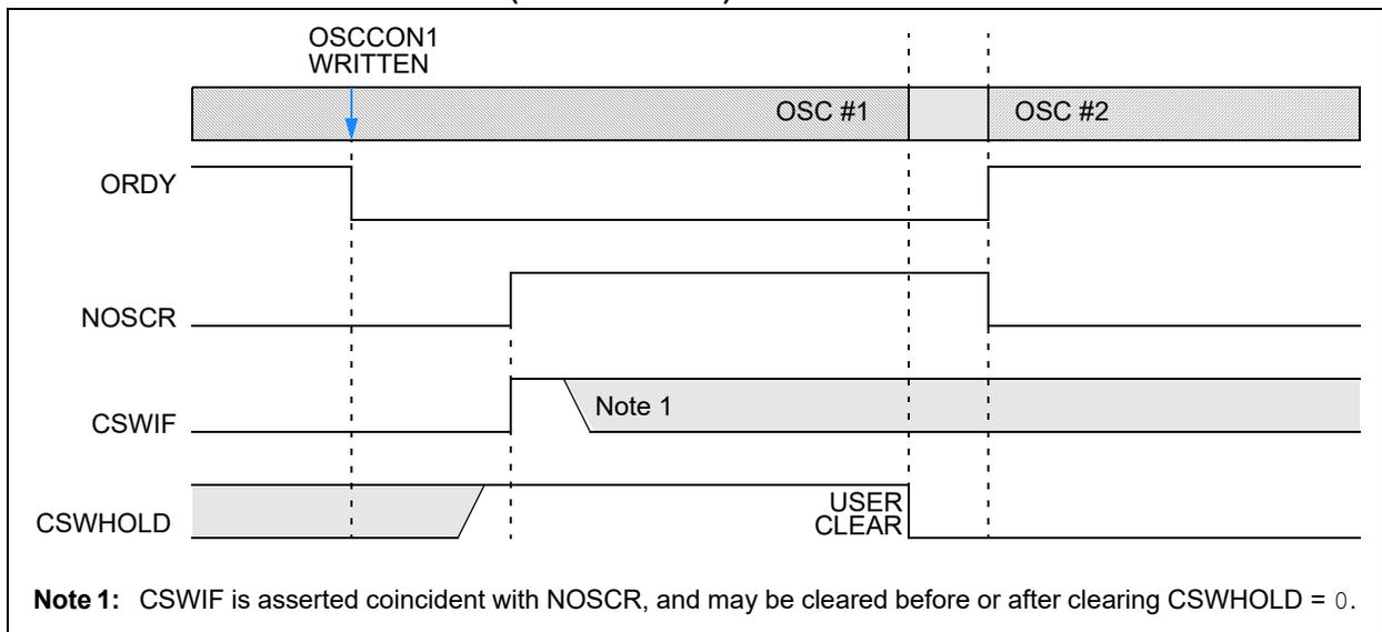
**FIGURE 7-8: CLOCK SWITCH ABANDONED**
