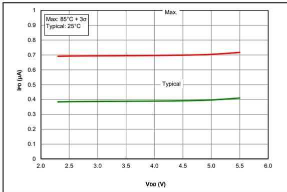
**FIGURE 36-15:**  $I_{PD}$  Base,  $V_{REGPM} = 1$ , (PIC16F18326/46 only)
