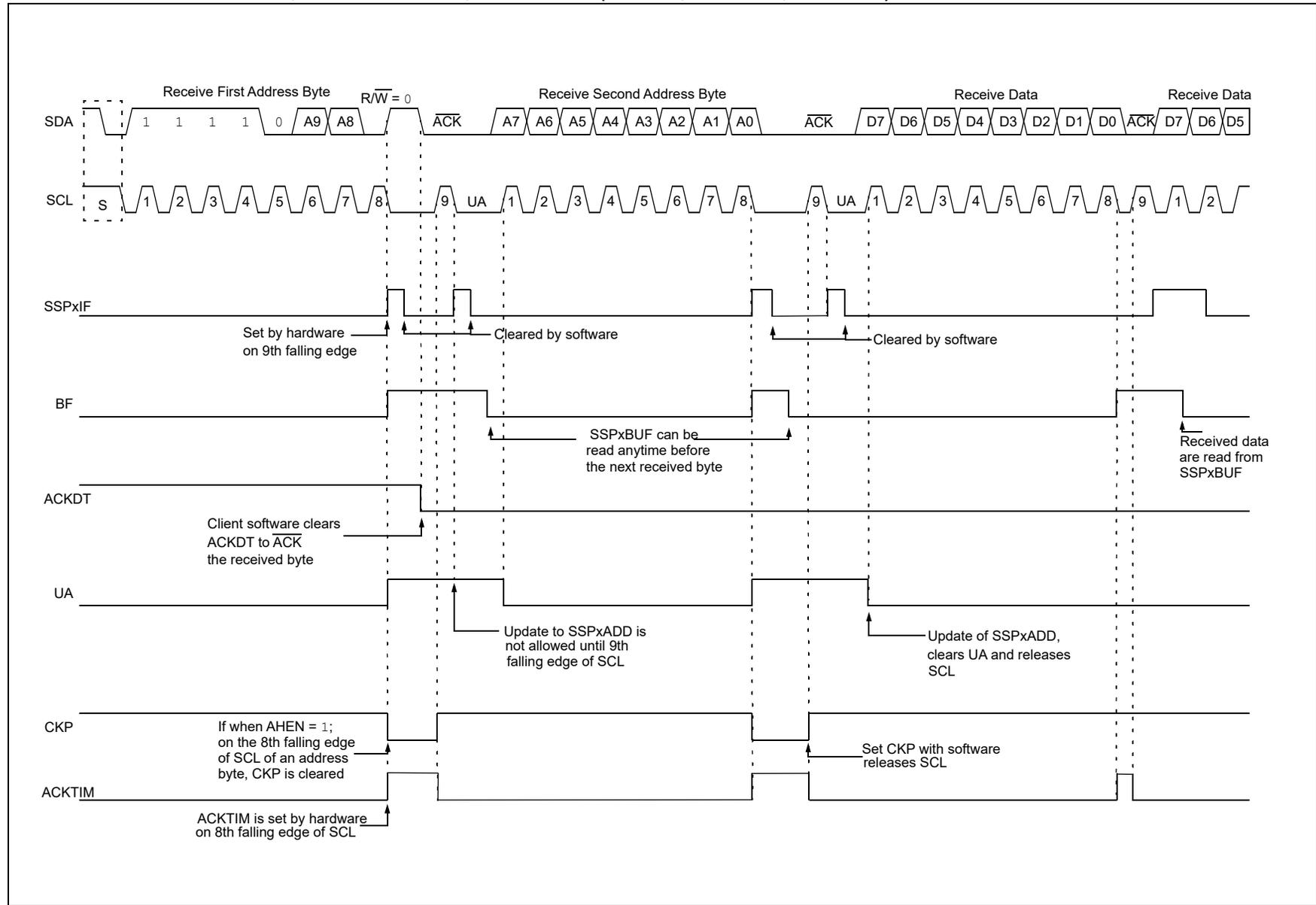
**FIGURE 30-22: I<sup>2</sup>C CLIENT, 10-BIT ADDRESS, TRANSMISSION (SEN = 0, AHEN = 0, DHEN = 0)**
