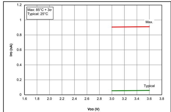
**FIGURE 36-10:**  $I_{PD}$ , Low-Power Brown-Out Reset ( $LPBOR = 1$ ) (PIC16LF18326/46 only)
