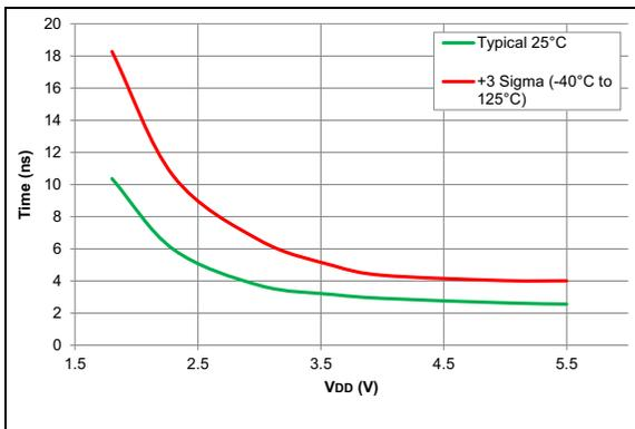
**FIGURE 36-107:** Rise Time, Slew Rate Control Disabled
