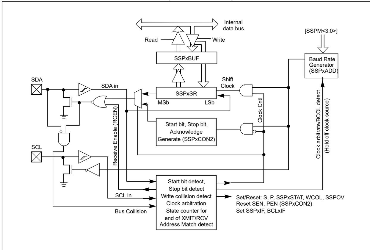
**FIGURE 30-3: MSSP BLOCK DIAGRAM (I<sup>2</sup>C CLIENT MODE)**
