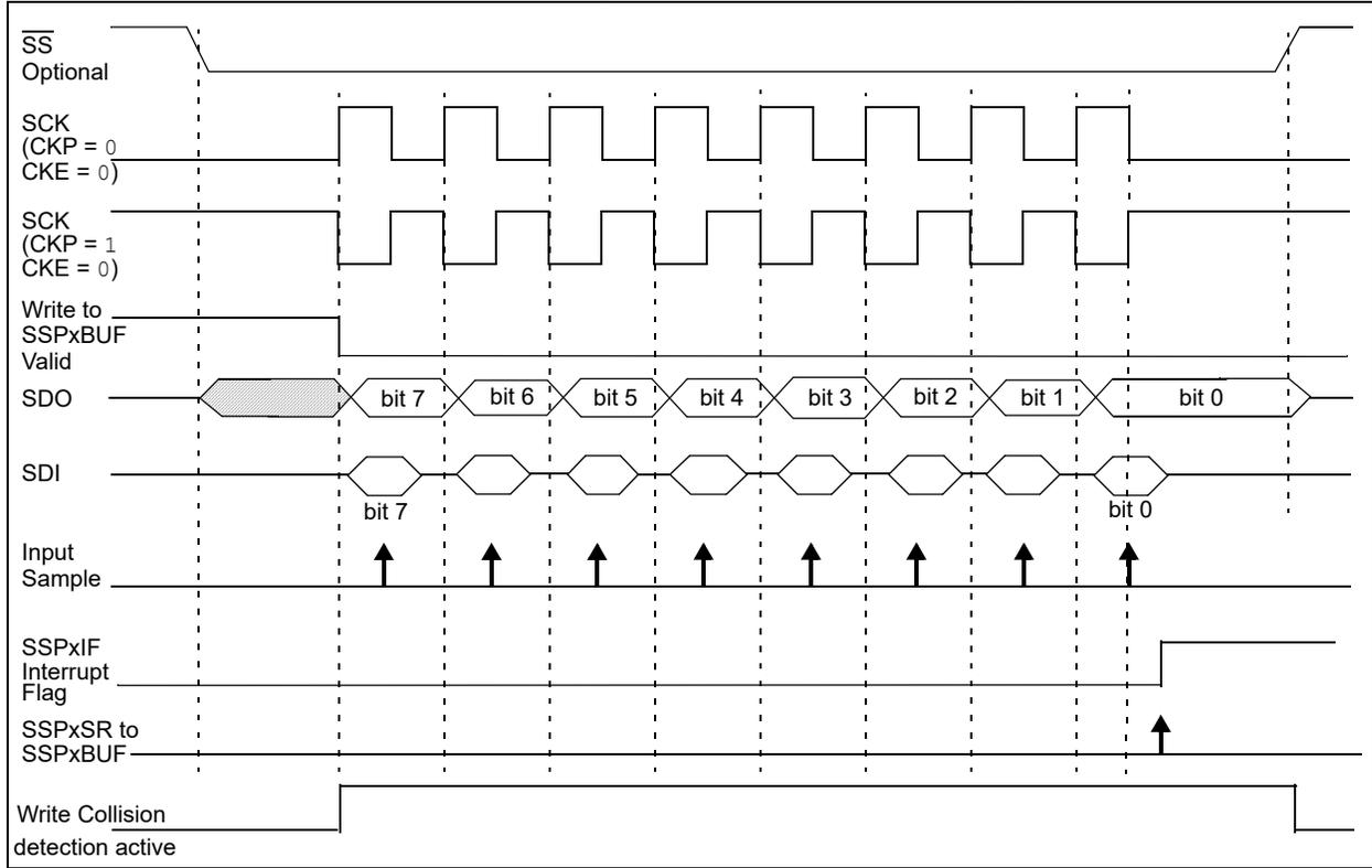
**FIGURE 30-10: SPI MODE WAVEFORM (CLIENT MODE WITH CKE = 1)**
