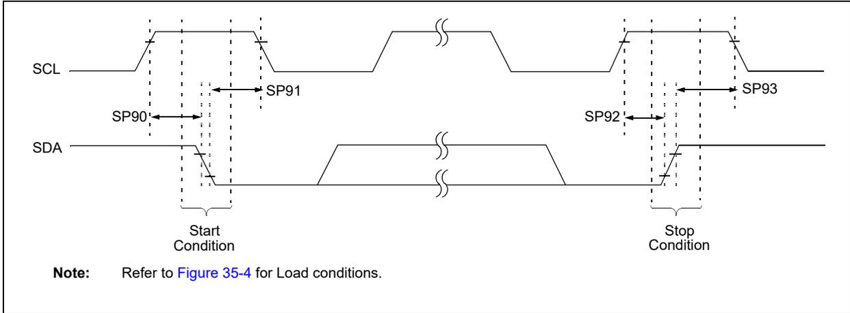
**TABLE 35-23: I<sup>2</sup>C BUS START/STOP BITS CHARACTERISTICS**
