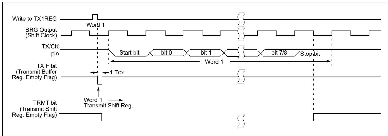
**FIGURE 31-4: ASYNCHRONOUS TRANSMISSION (BACK-TO-BACK)**
