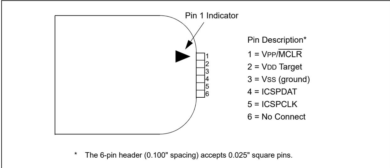
**FIGURE 33-3: TYPICAL CONNECTION FOR ICSP™ PROGRAMMING**
