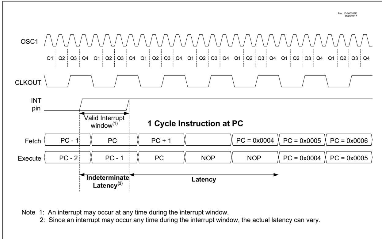
**FIGURE 8-3: INT PIN INTERRUPT TIMING**
