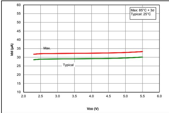
**FIGURE 36-7:**  $I_{PD}$ , Fixed Voltage Reference (FVR) (PIC16F18326/46 only)
