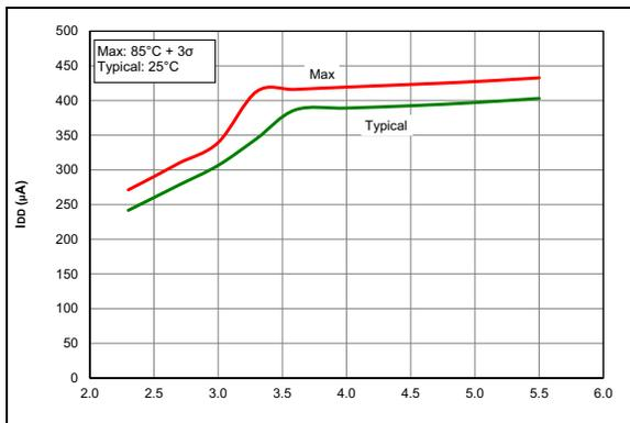
**FIGURE 36-17:**  $I_{DD}$ , XT Oscillator 4 MHz (PIC16F18326/46 only)
