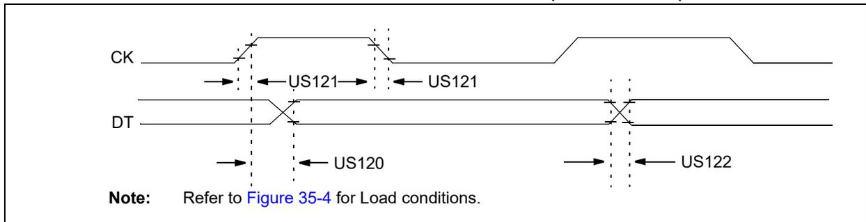
**TABLE 35-20: EUSART SYNCHRONOUS TRANSMISSION CHARACTERISTICS**
