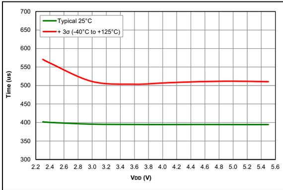
**FIGURE 36-117:** Wake From Sleep,  $V_{REGPM} = 1$  (PIC16F18326/46 only)
