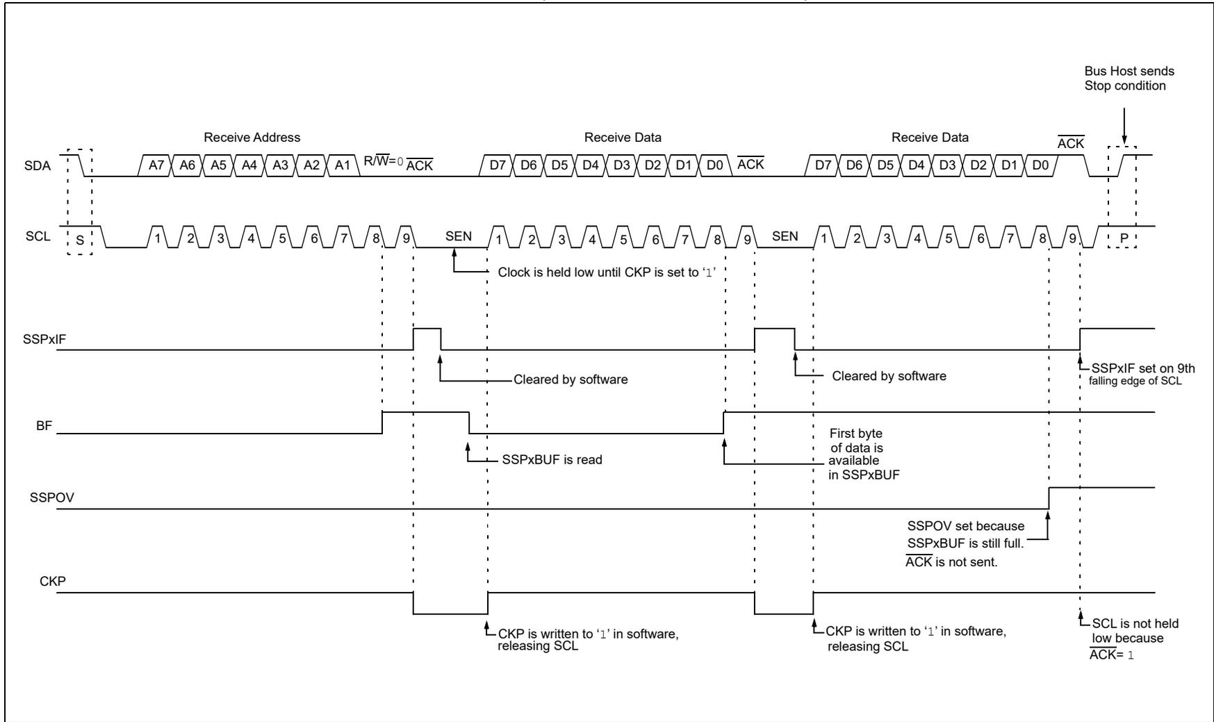
**FIGURE 30-16: I<sup>2</sup>C CLIENT, 7-BIT ADDRESS, RECEPTION (SEN = 0, AHEN = 1, DHEN = 1)**
