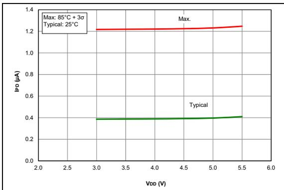
**FIGURE 36-11:**  $I_{PD}$ , Low-Power Brown-Out Reset ( $LPBOR = 0$ ) (PIC16F18326/46 only)
