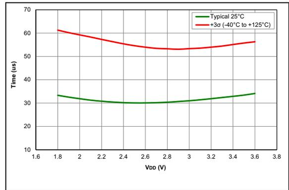
**FIGURE 36-94:** Band Gap Ready Time (PIC16LF18326/46 only)
