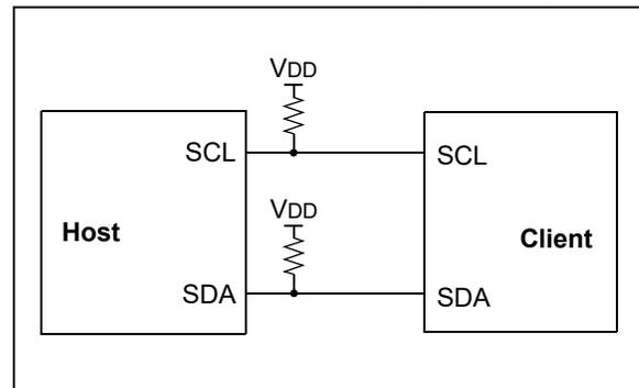
On the last byte of data communicated, the host device may end the transmission by sending a Stop bit. If the host device is in Receive mode, it sends a NACK in place of the last ACK bit. A Stop bit is indicated by a low-to-high transition of the SDA line while the SCL line is held high.
