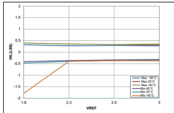
**FIGURE 36-60:** ADC 10-Bit Mode, Single-Ended INL,  $V_{DD} = 3.0V$ ,  $T_{AD} = 1\ \mu\text{s}$  (All devices)
