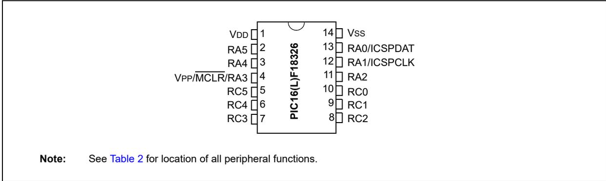
**FIGURE 2: 16-PIN UQFN/QFN/VQFN (4x4)**
