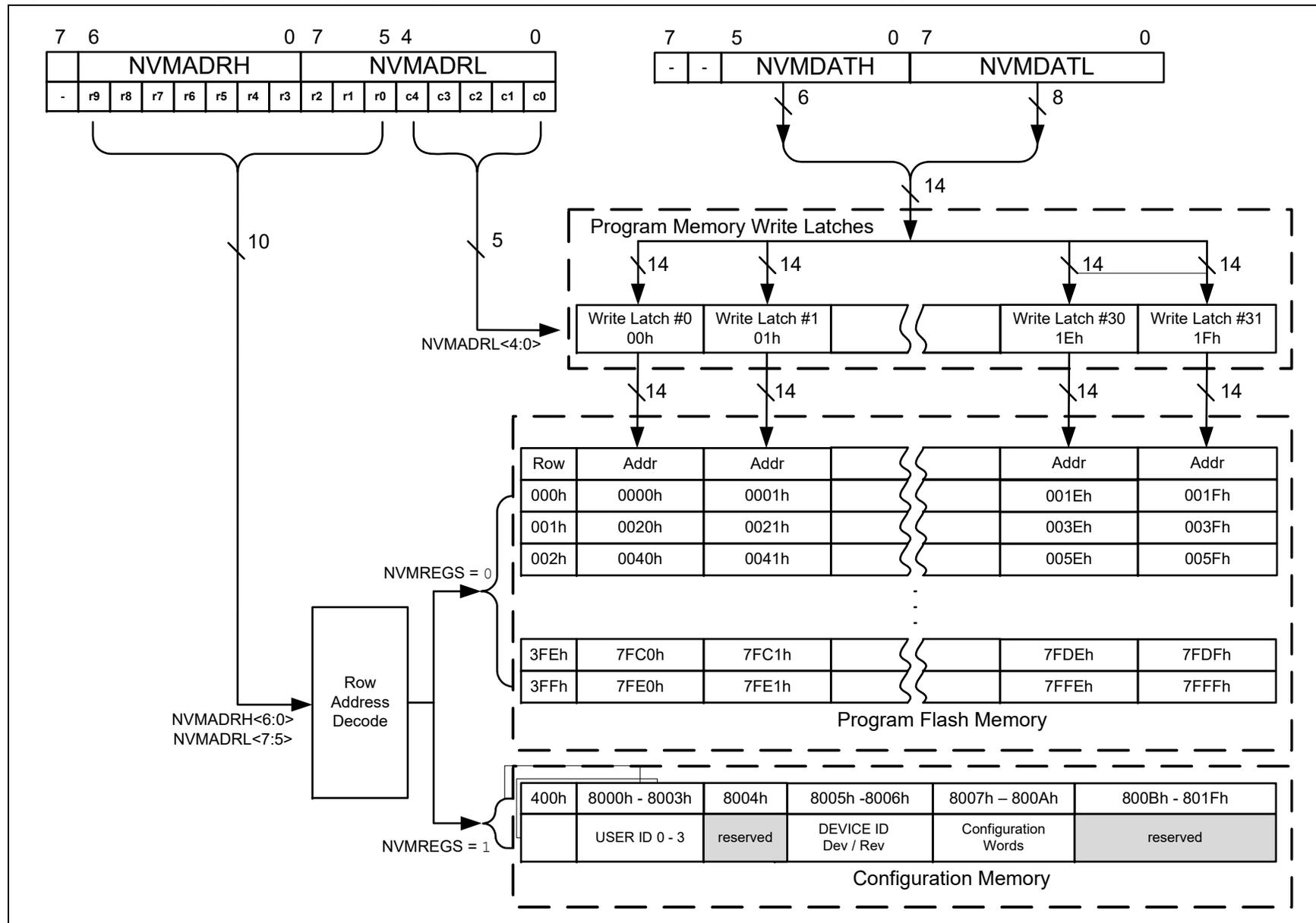
**FIGURE 11-5: PROGRAM FLASH MEMORY WRITE FLOWCHART**
