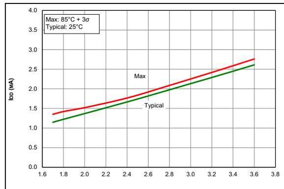
**FIGURE 36-18:**  $I_{DD}$ , HS Oscillator 32 MHz (PIC16LF18326/46 only)
