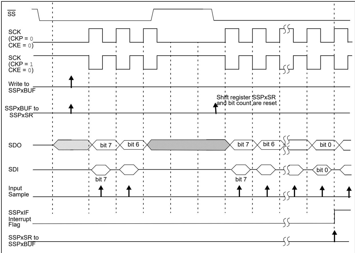
**FIGURE 30-9: SPI MODE WAVEFORM (CLIENT MODE WITH CKE = 0)**
