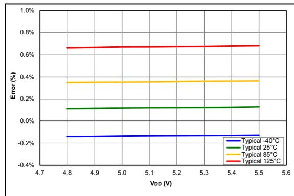
**FIGURE 36-100:** FVR Voltage Error 4x (PIC16F18326/46 only)
