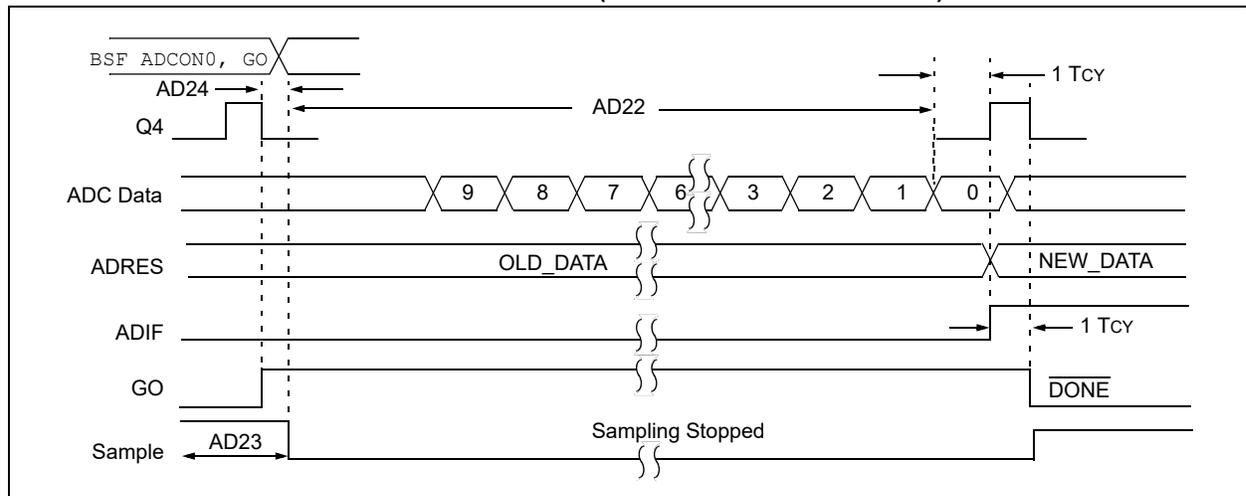
**FIGURE 35-11: ADC CONVERSION TIMING (ADC CLOCK FROM ADCRC)**
