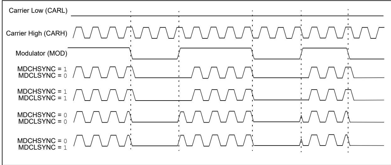
**FIGURE 25-3: NO SYNCHRONIZATION (MDSHSYNC = 0, MDCLSYNC = 0)**
