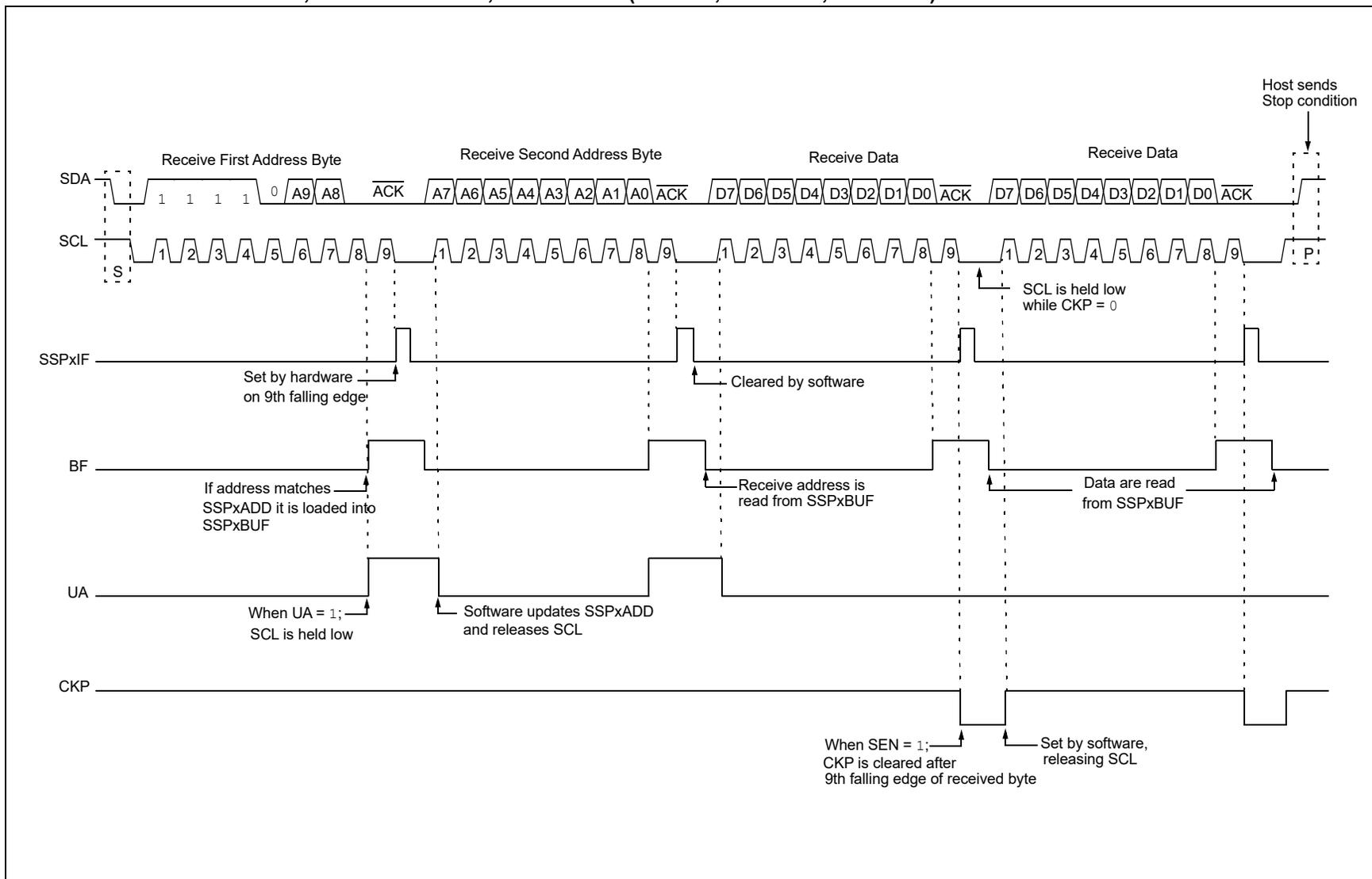
**FIGURE 30-21: I<sup>2</sup>C CLIENT, 10-BIT ADDRESS, RECEPTION (SEN = 0, AHEN = 1, DHEN = 0)**
