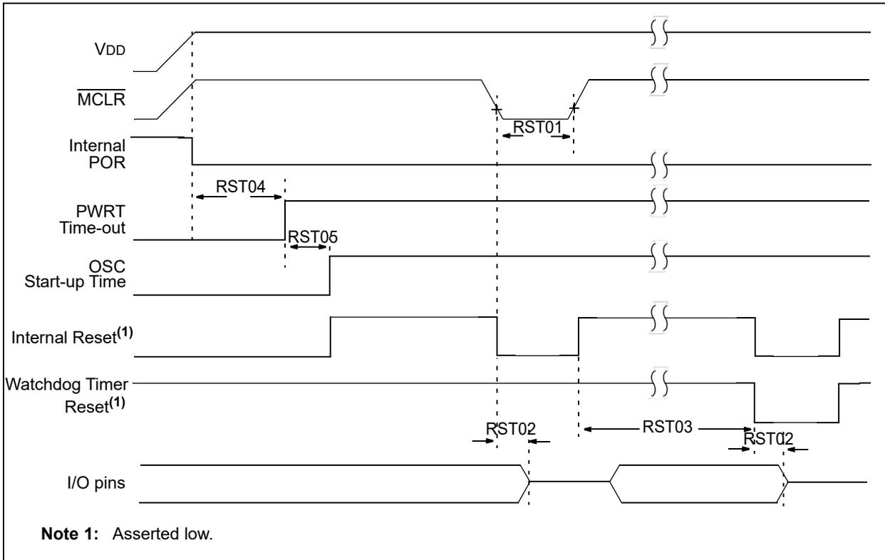
**FIGURE 35-9: BROWN-OUT RESET TIMING AND CHARACTERISTICS**
