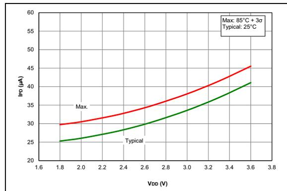
**FIGURE 36-6:** IPD, Fixed Voltage Reference (FVR) (PIC16LF18326/46 only)
