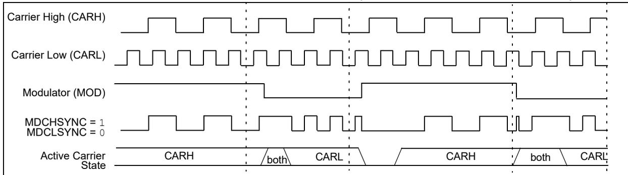
**FIGURE 25-5: CARRIER LOW SYNCHRONIZATION (MDSHSYNC = 0, MDCLSYNC = 1)**
