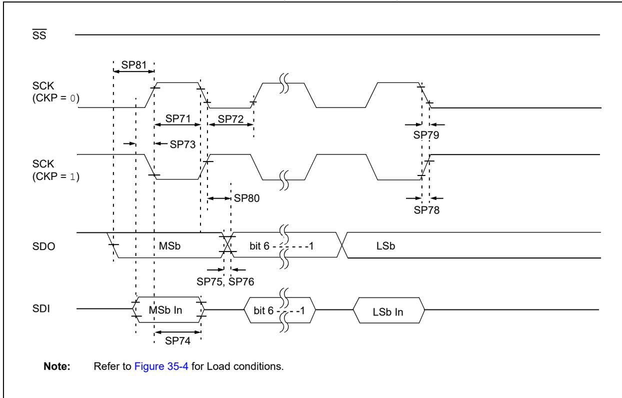
**FIGURE 35-19: SPI CLIENT MODE TIMING (CKE = 0)**
