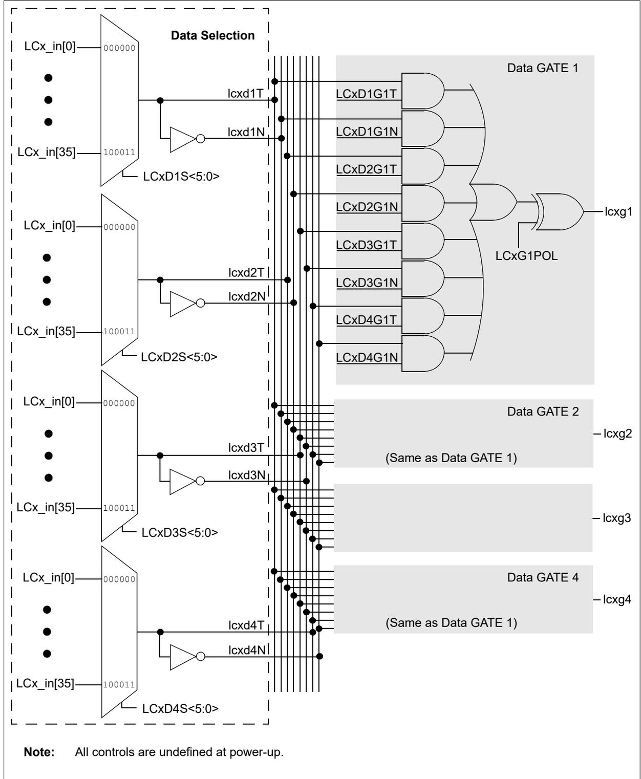
**FIGURE 21-3: PROGRAMMABLE LOGIC FUNCTIONS**
