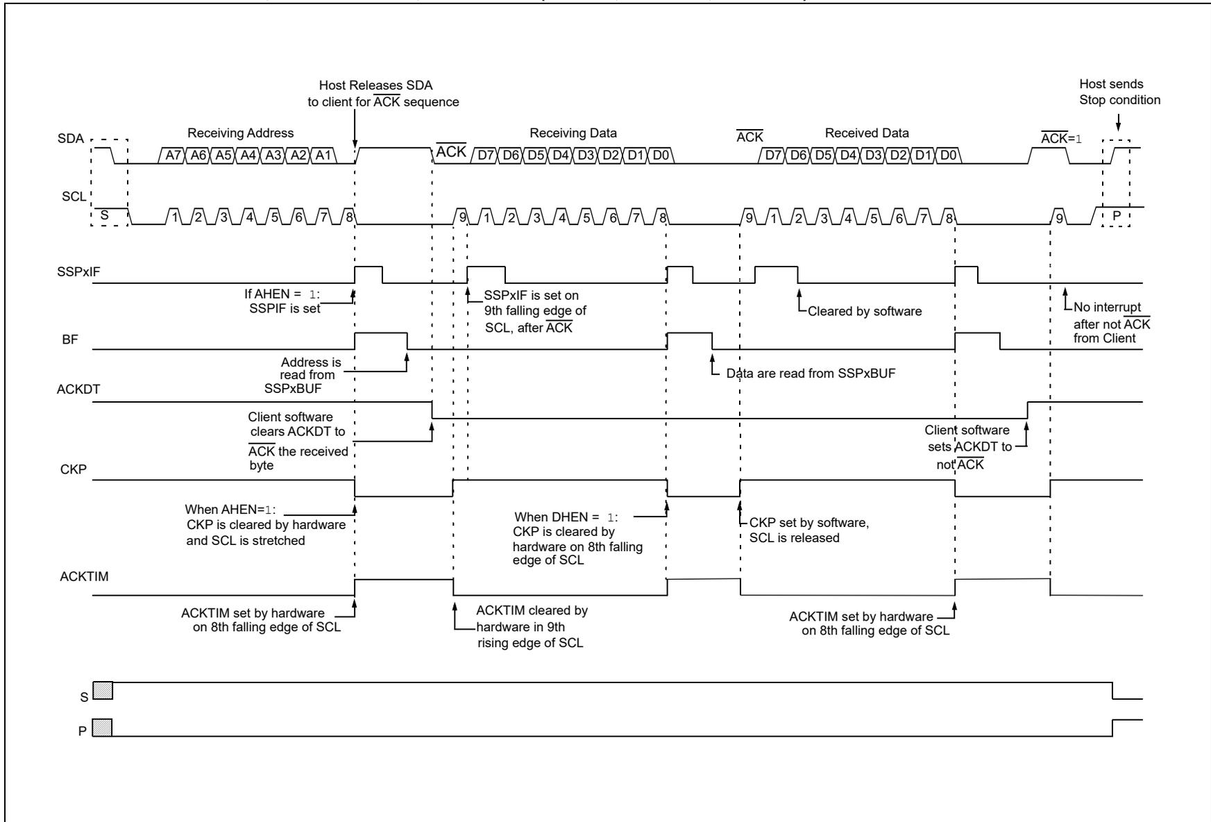
**FIGURE 30-17: I<sup>2</sup>C CLIENT, 7-BIT ADDRESS, RECEPTION (SEN = 1, AHEN = 1, DHEN = 1)**
