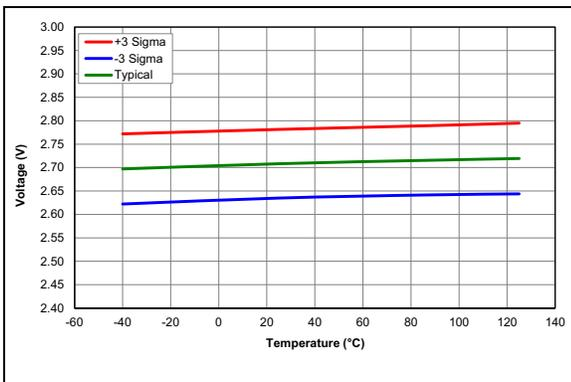
**FIGURE 36-41:** Brown-Out Reset Voltage,
