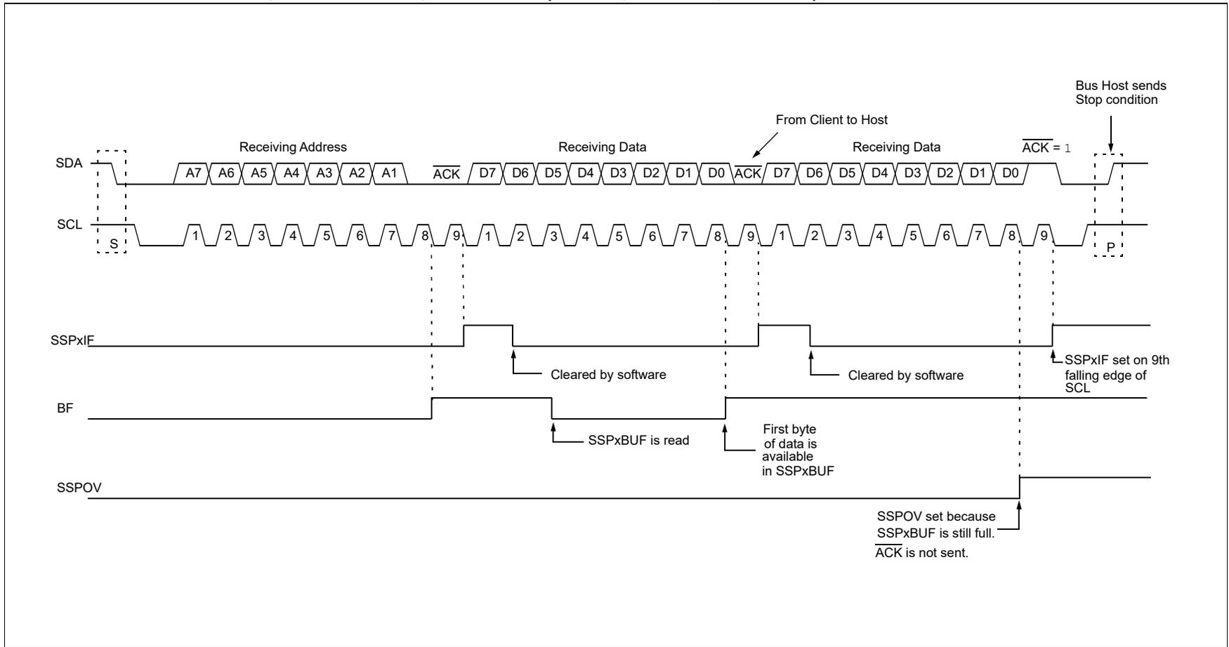
**FIGURE 30-15: I<sup>2</sup>C CLIENT, 7-BIT ADDRESS, RECEPTION (SEN = 1, AHEN = 0, DHEN = 0)**
