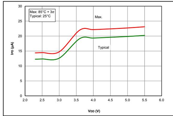
**FIGURE 36-14:**  $I_{PD}$  Base,  $V_{REGPM} = 0$ , (PIC16F18326/46 only)
