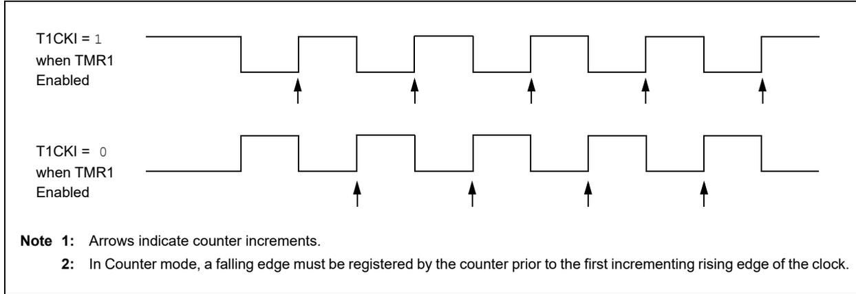
**FIGURE 27-4: TIMER1 GATE ENABLE MODE**
