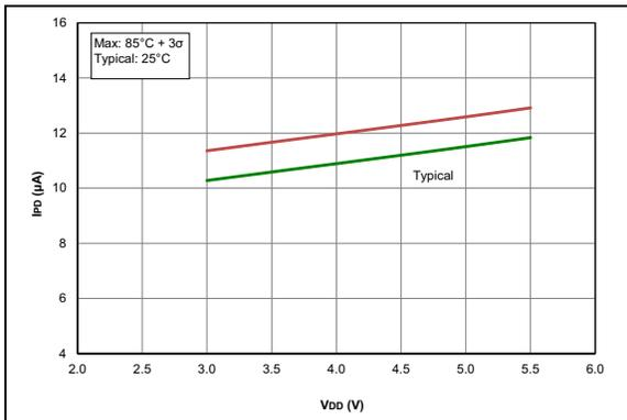
**FIGURE 36-9:**  $I_{PD}$ , Brown-Out Reset (BOR),  $BORV = 1$  (PIC16F18326/46 only)
