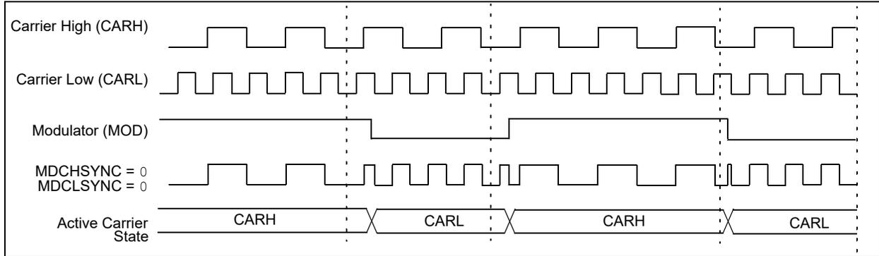
**FIGURE 25-4: CARRIER HIGH SYNCHRONIZATION (MDSHSYNC = 1, MDCLSYNC = 0)**
