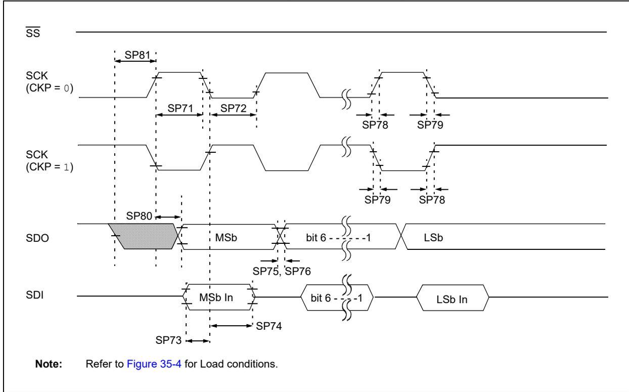
**FIGURE 35-18: SPI HOST MODE TIMING (CKE = 1, SMP = 1)**
