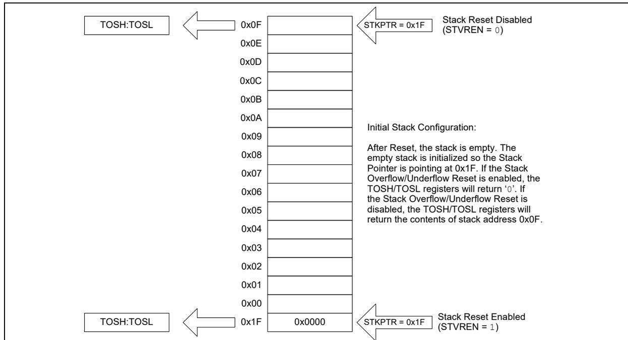
**FIGURE 4-5: ACCESSING THE STACK EXAMPLE 2**
