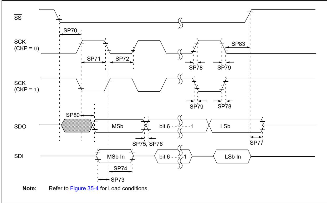
**FIGURE 35-20: SPI CLIENT MODE TIMING (CKE = 1)**
