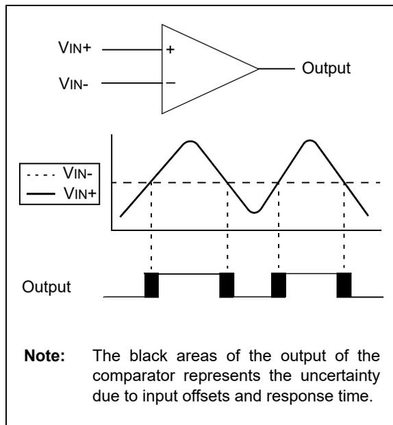
**FIGURE 19-2: COMPARATOR MODULE SIMPLIFIED BLOCK DIAGRAM**
