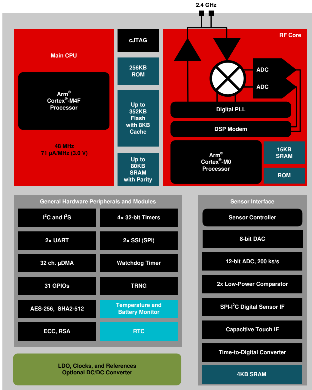
Figure 4-1. CC2662R-Q1 Block Diagram
